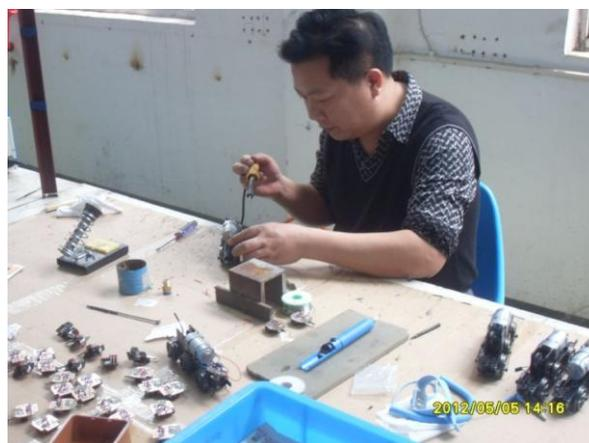
**3: Mechanisms are tested again but this time with the PCB and the switches on them. The mechanisms should start running slowly at 3 Volts but this particular one starts at 1.7 Volts as can be seen. After the body is assembled the complete engine will be run again before packing. We have put foam underneath the rails so I can concentrate on hearing the sound of the mech. When a mechanism zooms by there is little to see or to inspect but the sound will reveal any defect.**
