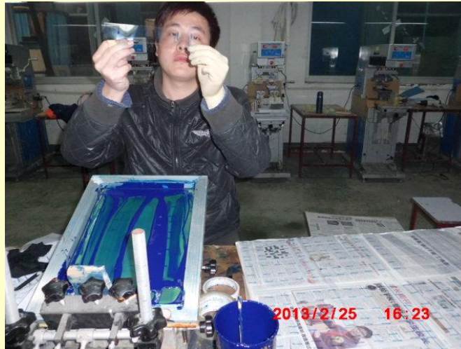
Screen printing the coach window glazing.
