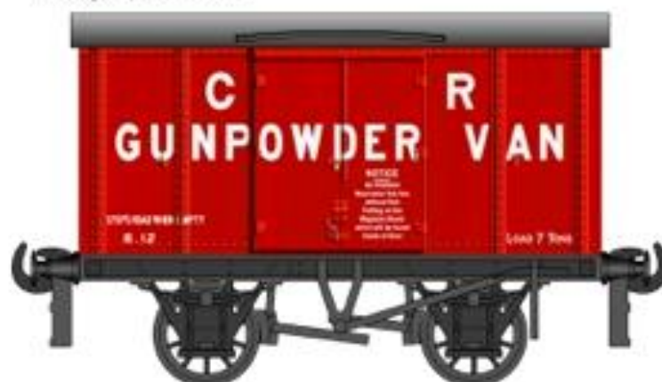
Caledonian Railway gunpowder van built around 1915. The notice on the door of the van states that anyone entering the vehicle must wear the magazine boots provided so as to reduce the risk of an explosion caused by sparks from 'hobnail' boots.
