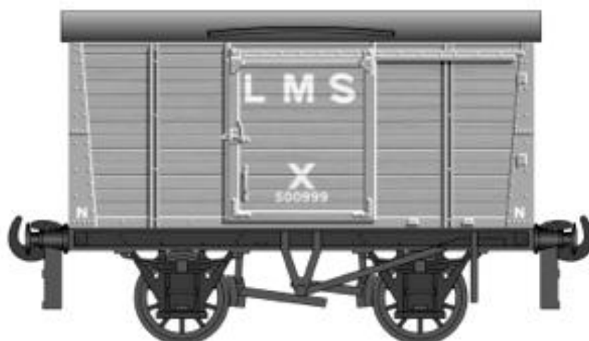
LMS 12 Ton ventilated van. This varies from the other two (below) in that it has different "wrap around" steel corners and exterior vertical channel strapping. Circa 1934-5
