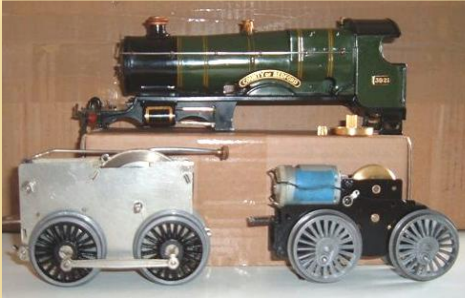
An example of a large Hornby loco with original clockwork mechanism (left) and new 'Toys of the Past' electric mechanism (right)
