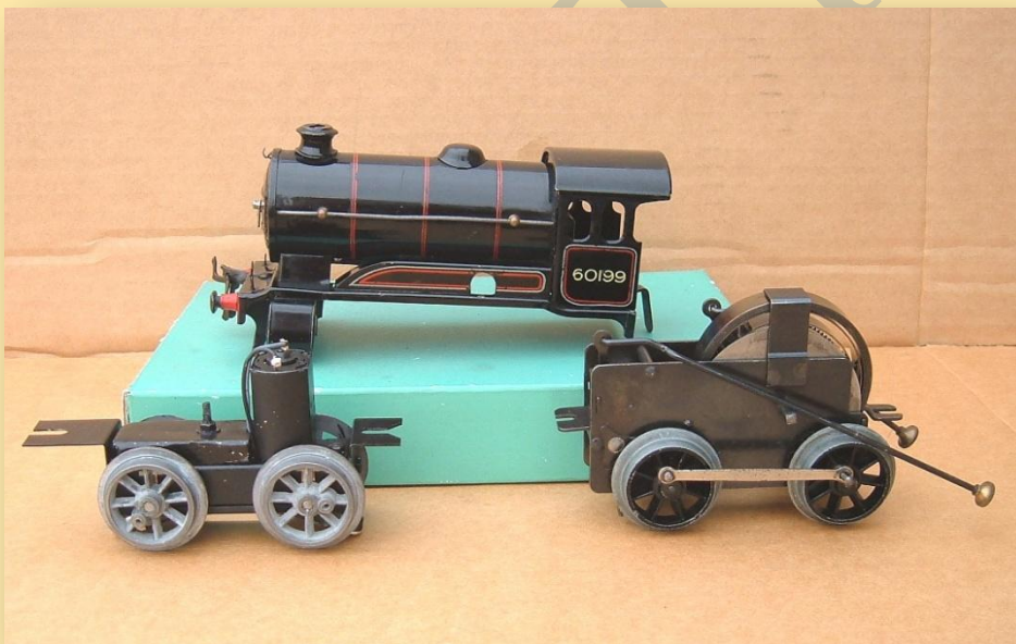
An example of a small Hornby loco with original clockwork mechanism (right) and new 'Toys of the Past' electric mechanism (left)
