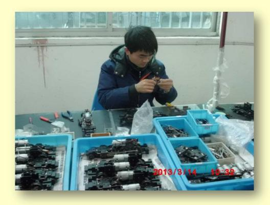
Here, the Castle switch wiring is being soldered.
