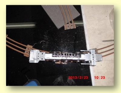
Below is another recently released photograph from the factory. This is the first view of the two rail version of the six wheel drive mechanism, the red arrow identifying the newly devised electrical contact strip.
