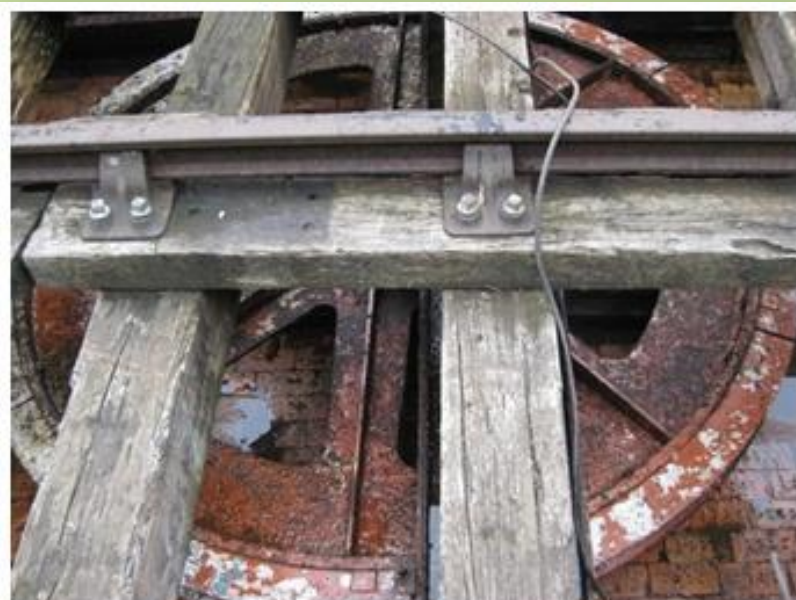
Looking down on the large horizontal winding wheel at the foot of the incline.
