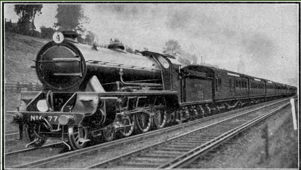
Photo]. Down "Atlantic Coast Express" in Clapham Cutting, Southern Railway. 4-6-0 engine No. 775 "Sir Agravaine," of the "King Arthur" class with latest type of cab and tender [F. E. Mackay
